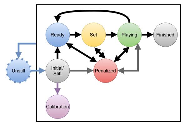
Figure 7: Diagram of the robot states.
