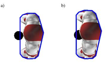
Figure 10: Examples for "Ball Holding". The black circle is the ball, the blue polygon visualizes the convex hull of the robot's projection onto the ground and the red area shows the occupied portion of the ball. Situations a) is legal, whereas b) violates the rule.
