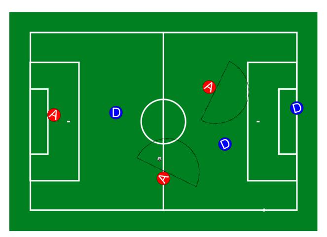
Figure 20: Possible challenge situation with attacking robots already oriented towards their targets. The arcs for a valid pass are indicated with dashed line style.
