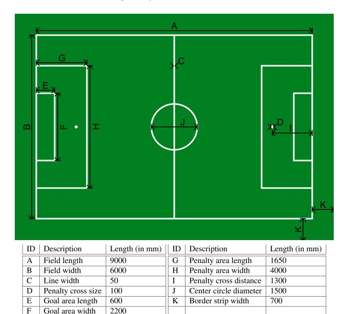
Figure 1: Schematic diagram of the soccer field (not to scale) and corresponding dimensions in mm. Note that measurements on this diagram are made to the center of lines.
