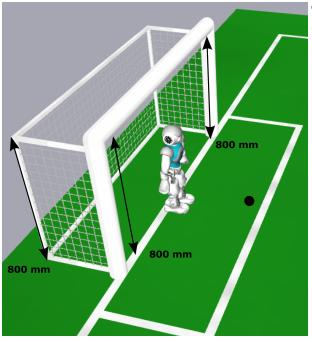
The goalposts and crossbar are made from 3 white cylinders with a diameter of 100 mm. The net:
